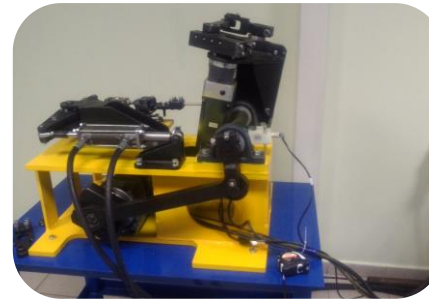
Endurance tests of car racks
