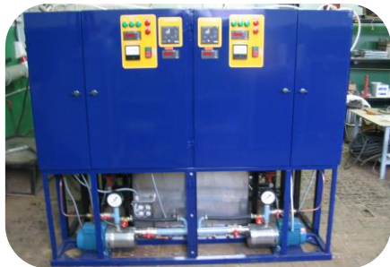
Steam generators for drilling rigs
