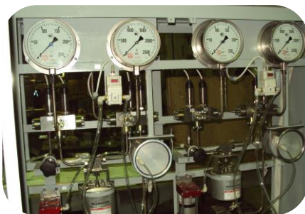
Overpressure testing of parts
