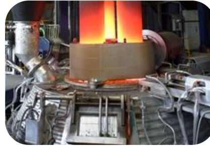
Ladle furnaces (15-375 tons)
