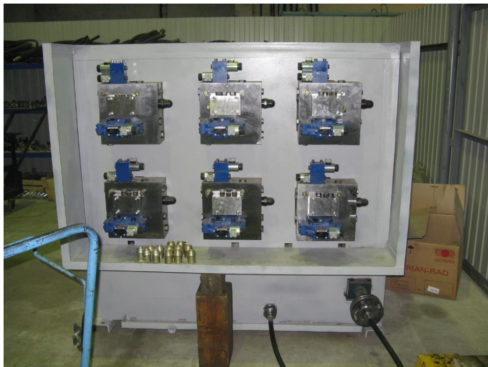
Hydropanel for control of shut-off control valves of the main hydraulic control valve
