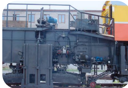
Hydraulic equipment of lining, trimming and leveling machines
