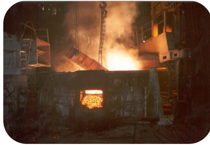
Arc furnaces (6-120 tons)
