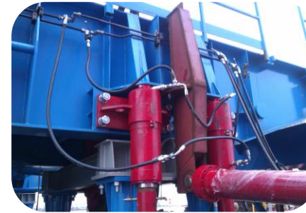
Drilling rig moving and leveling system
